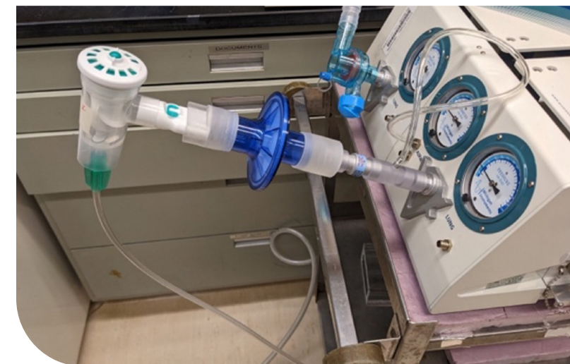
Dr. Mainelis (Rutgers University) and colleagues developed a custom experimental approach that utilizes a lung simulator to assess nebulizer characteristics.
